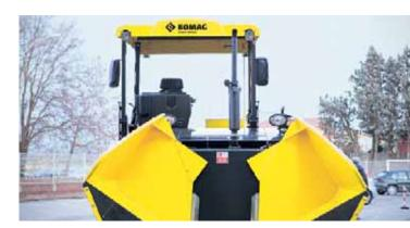
A change of perspective: the BOMAG SIDEVIEW system gives a lateral overhang of up to 40 cm.
