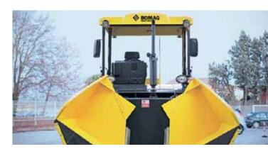
With the BOMAG SIDEVIEW system, the finisher needs just one seat and one operating console.
