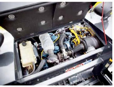
High power, low consumption: the Kubota engine in the BF 300 finisher.
