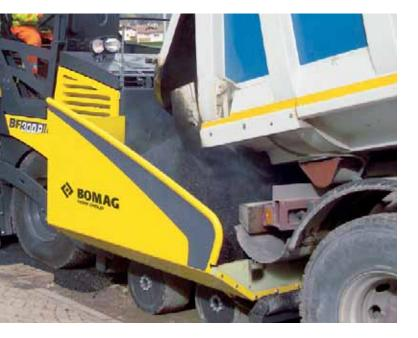
The amply-sized hopper opening makes re-charging from trucks quick and easy.
