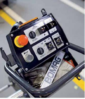
User focus: the rotating side-mounted operator's station with ample shelf space.
