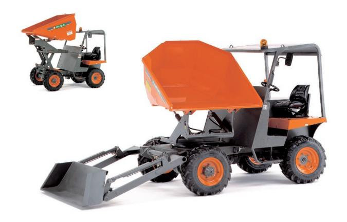
2,5/3 ton rigid chassis dumper with mechanical or hydrostatic transmission. Great skip capacities from 1.200 to 1.950 l. High stability in rough terrain.
