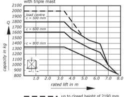
— — — up to closed height of 2190 mm over closed height of 2240 mm
